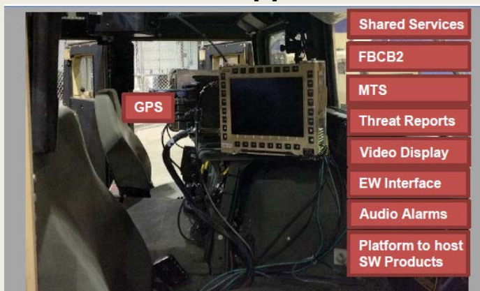
VICTORY Data Bus enables interoperability across C4ISR/EW and platform systems
